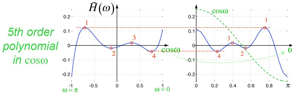
$\Rightarrow \tilde{H}(\omega)$  has at most  $M-1$  min/max (ripples)
